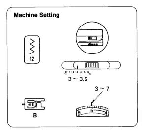
Tape the button over the placement mark. A pin can be placed on top of the foot to from a shank. Before lowering the foot, test the needle swing making sure the needle drops in each hole.
