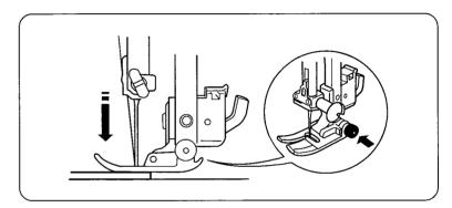
Lower the needle into the fabric at the point where you wish to start sewing. Press the small black button on the zigzag foot with your left hand to "lock" the presser foot to the fabric.
