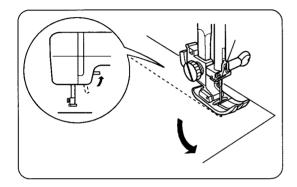
Stop the machine and bring the needle down into the fabrics by pressing Up/Down needle position button.
