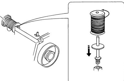
Lift up the spool pin. Place the spool of thread on the spool with the thread coming off the spool as shown.
