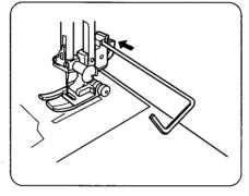
The quiliting guide will help to keep the stitchintg lines straight. Insert the quilter in the opening, and slide it at the desired width.
