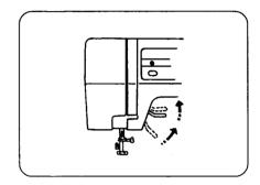
The presser foot can be raised higher for additional clearance.
