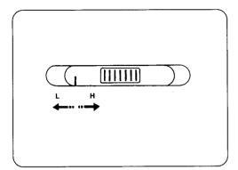
The maximum sewing speed can be controlled by the speed setting lever. To increase the speed, slide the lever to the right.
