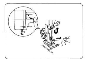
② Press the Up/Down needle position button twice to pick up the bobbin thread.
