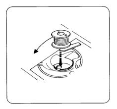
Place the bobbin in the bobbin holder with the thread running counter-clockwise.
