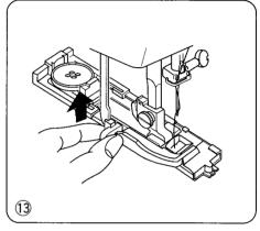
(13) When buttonhole sewing is finished, push the buttonhole lever upward as far as it will go.
