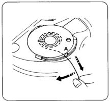
Guide the thread into the notch **A** on the front side of the bobbin holder. Draw the thread to the left sliding it between the tension spring blades.
