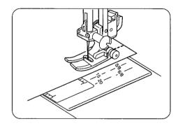
The numbbers on the needle plate indicate the distance between the left needle position and the line.
