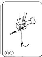
Press the Up/Down needle position button to raise the needle to its highest position. Raise the presser foot with the presser foot lifter and thread in the order from ① to ⑤.
