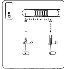
When pattern number 13 is selected, you can move the needle between center and left needle positions.
