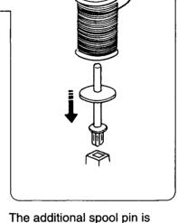
used to wind extra bobbins without unthreading the machine.
