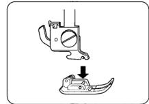
When attaching the presser foot, the pressure dial should always be at position "3". Place the presser foot so the pin on the foot lies just under the groove of the foot holder. Lower the foot holder to lock the foot in place.
