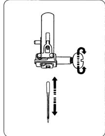
Loosen the needle clamp screw by turning it counter-clockwise.
