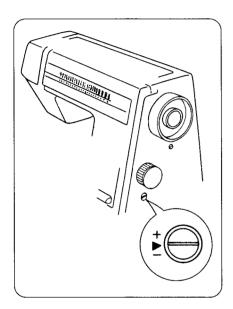
If patterns are uneven when sewing with a particular fabric, adjust them with the feed balance dial.
