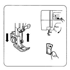
Raise the needle bar by pressing Up/Down needle position button and lower the presser foot. Turn off the power switch.
