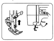
Press the Up/Down needle position button to raise the needle to its highest position. Raise the presser foot.
