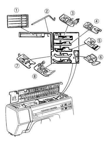
Each presser foot and pocket is lettered for easy identification and storage. To achieve optimum sewing results, use the foot recommended for each sewing technique.
