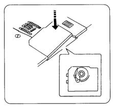
Pull out about 15 cm (6") of thread and attach the hook cover plate.
