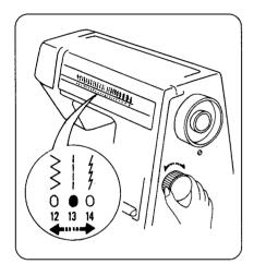
Select the pattern by turning the pattern selector dial and the red signal (LED) shows the selected pattern.
