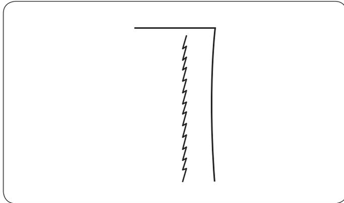
This stitch is a narrow stretch stitch designed to eliminate puckering on knit fabrics and bias seams, while permitting the seam to be pressed completely open flat. Use this stitch for seaming fine fabrics.
