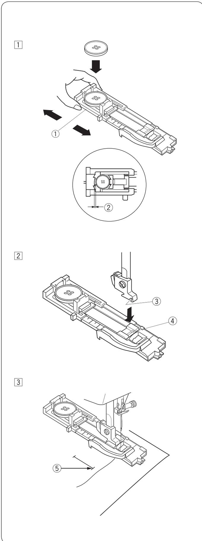
The size of a buttonhole is automatically set by placing a button in the rear of automatic buttonhole foot R. The button holder of the foot takes a button size of 3/8" (1 cm) to 1" (2.5 cm) in diameter. When selecting the buttonholes, the LCD display advise you to lower the buttonhole lever.
