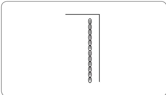
This strong, durable stitch is recommended when both elasticity and strength are necessary in order to insure comfort and durability. Use it to reinforce areas such as crotch and armhole seams. Also use for extra reinforcement when constructing items such as backpacks.
