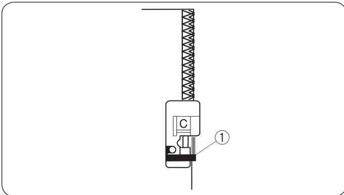
This stitch is excellent for sewing fabrics that tend to fray extensively such as linens and gabardines. Two rows of zigzag stitches are simultaneously sewn over the edge to insure that your seams will not ravel. Sew while guiding the fabric edges along the guide on the foot.
