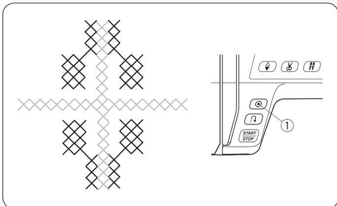
Use a plain close woven fabric such as linen or wool flannel. If you use light weight fabric, apply a tear away backing for support.
