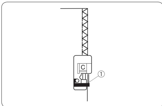
This stitch is used to seam and overcast fabric edges at one time.
