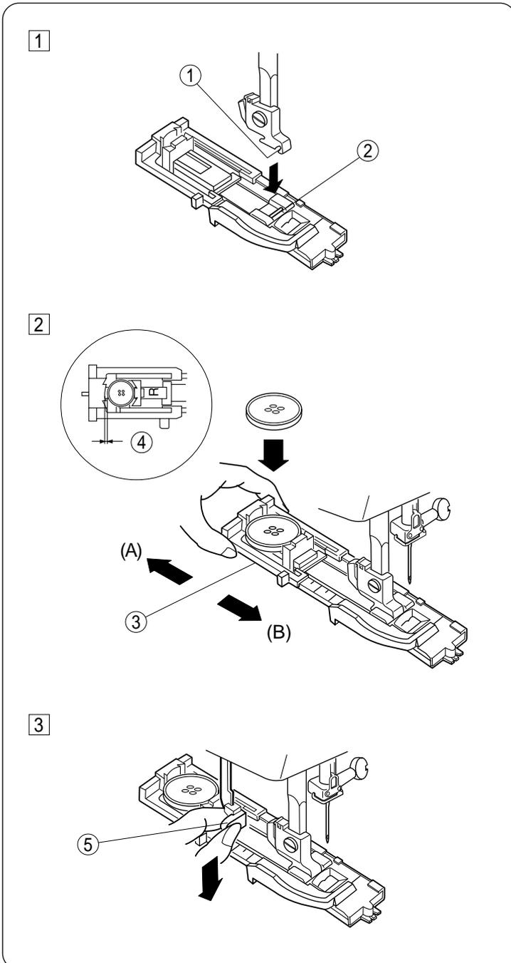
① Raise the needle and foot. Place the automatic buttonhole foot with its pin just under the groove of the foot holder. Lower the presser bar to attach the automatic buttonhole foot.
