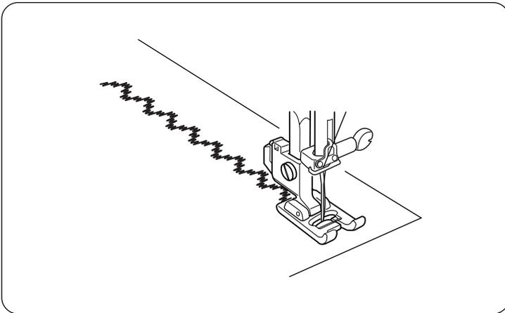
Test the stitch on the actual fabric for the desired patterns and adjust the stitch density for the best sewing results.
