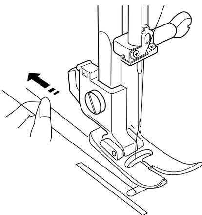
3 Draw 10 cm (4") of both threads to the back under the presser foot.
