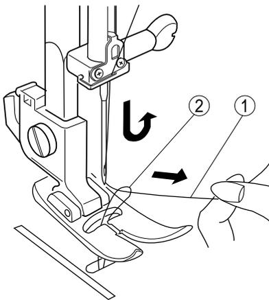
2 Turn the handwheel one complete rotation toward you and raise the needle to its highest position. Pull the needle thread to pick up a loop of the bobbin thread.
