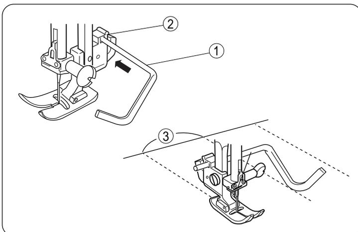
Insert the quilting bar into the opening on the back of the foot holder.
