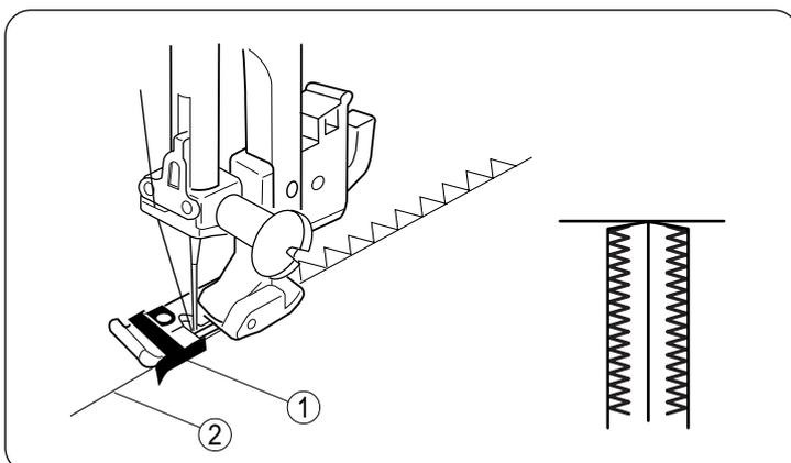
**CAUTION:** Do not set the stitch width less than 5 when using the overedge foot to prevent the needle from hitting the wires on the foot.
