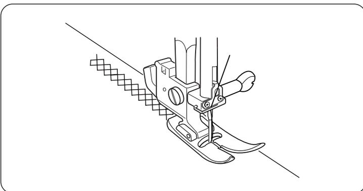
As the fabric moves back and forth in the stretch stitch sewing, guide the fabric carefully to keep the seams straight.
