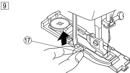
4 Draw the needle thread to the left through the hole on the foot. Place the fabric under the foot and lower the needle at the starting point of the buttonhole mark. Then lower the foot.
