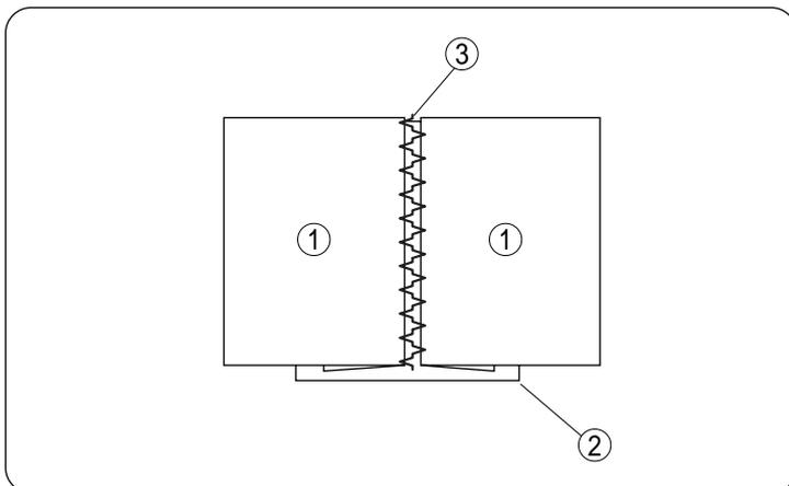
1. Fold under 1.5 cm (1/2") on each fabric edge and press. Pin the two edges to a piece of paper 0.3 cm (1/8") apart.
