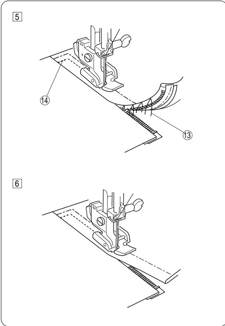
5 Detach the foot and re-attach it with the pin on the left. Backstitch across the end of opening to 0.7 – 1 cm (3/8"). Turn the fabric 90 degrees and stitch through the garment and zipper tape. Stop the machine 5 cm (2") before the foot reaches the slider on the zipper tape. Lower the needle into the fabric, and raise the foot. Remove the basting stitches.
