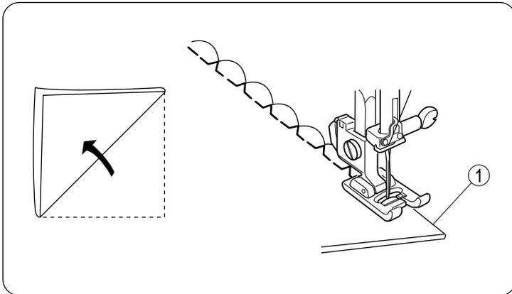
Fold the fabric in bias. Sew along the folded edge so that the needle on the right swing just clear the folded edge to form tucks.
