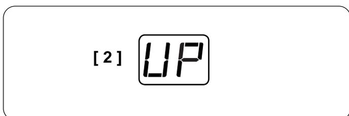
[2] If you select the other pattern without raising the presser foot or buttonhole lever, the LED display shows "UP". Select the other pattern after raising the foot and buttonhole lever.
