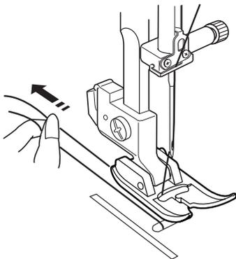
1 Raise the presser foot. Hold the needle thread lightly with your left hand.
