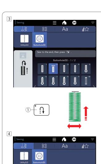
3 Start sewing again, and the machine sews the front bartack and right side of the buttonhole.
