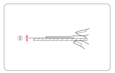
To check needle straightness, place the flat side of the needle onto something flat (a needle plate, glass etc.).
