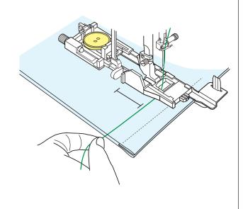
3 Place the fabric between the buttonhole foot and stabilizer plate. Lower the needle into the starting point by turning the handwheel.
