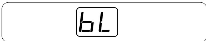
If you start sewing the buttonhole without lowering the buttonhole lever, the indicator will show a warning sign. Lower the buttonhole lever, then restart the machine.
