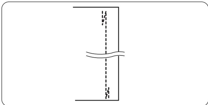
This reverse stitch can be used for securing, mending or reinforcement stitches. At the end of seams, press the reverse stitch button ④ once, so that the machine will sew an auto-lock stitch immediately and stop automatically.
