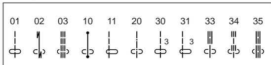
When you select stitch patterns above, you can adjust the left/right needle position. When you press “-”, the needle position will move to the left. When you press “+”, the needle position will move to the right.
