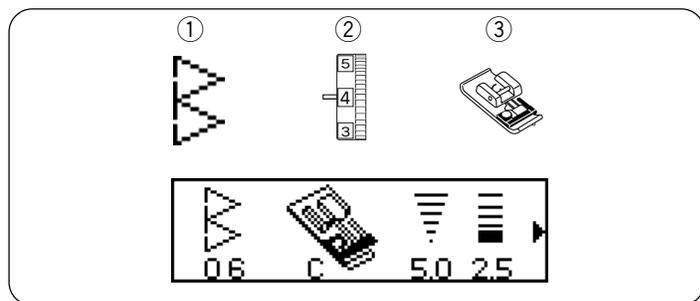
This stitch pattern combines the straight and the zigzag stitches, using the overedge foot, to stitch and overcast seams in one step.
