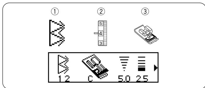
This stitch can be used for sewing fabrics that tend to fray extensively such as linens and gabardines.
