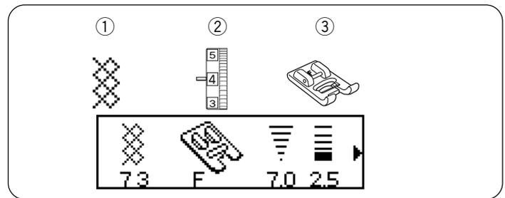
**NOTE:** Loosen the needle thread tension to make gathering easier.
