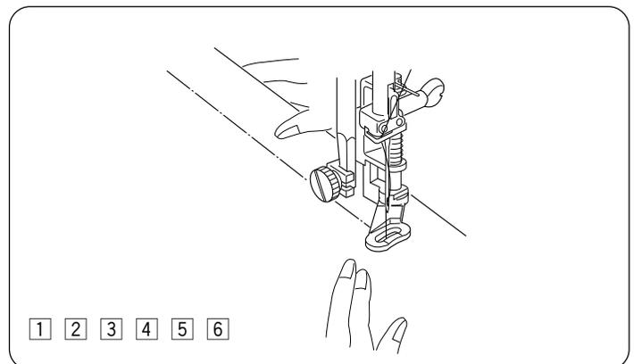
\* After sewing, reset tension to "4". Return feed dog lever to raised position. Feed dog will rise when sewing resumes.
