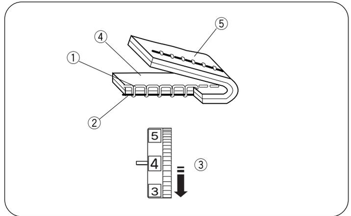
**Adjust the needle thread tension for a zigzag stitch**
