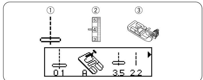
Place the folded fabric under the raised presser foot. Lower the needle into the fabric 1/16" (0.1 to 0.2 cm) from the folded edge. Lower the presser foot. Turn the screw to adjust the guide on the blind hem foot to touch the folded fabric edge.
