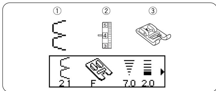
Use a lightweight fabric (tricot, for example). Fold the fabric as shown and stitch on the fold. Allow the needle to just clear the folded edge to create a shelled edge. You may need to increase the needle thread tension slightly.
