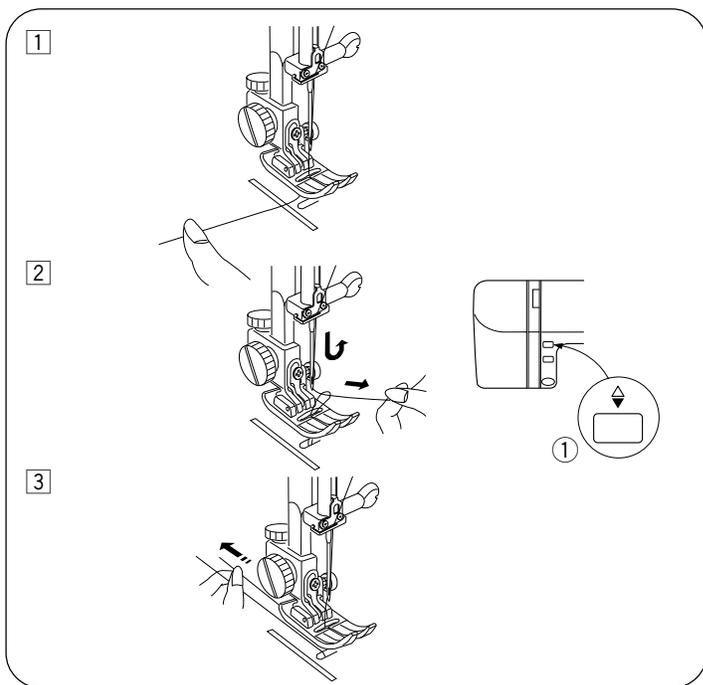
**Adjust the needle thread tension for a straight stitch**
