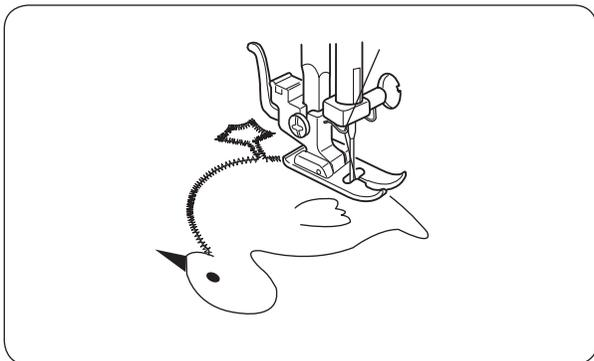
Baste (or fuse with iron-on fabric joiner) applique pieces on the fabric. Stitch around the applique making sure the needle falls along the outer edge of the applique. When sewing corners, lower the needle down into the fabric. Raise the presser foot and pivot the fabric to the right or left.
