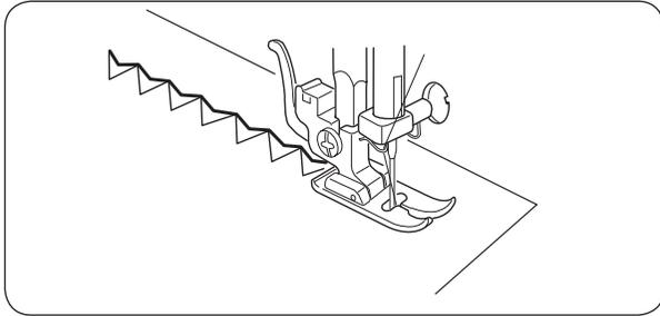
If forward and reverse feeds become unbalanced due to the type of fabric, adjust the balance by turning the stitch length dial as follows:
