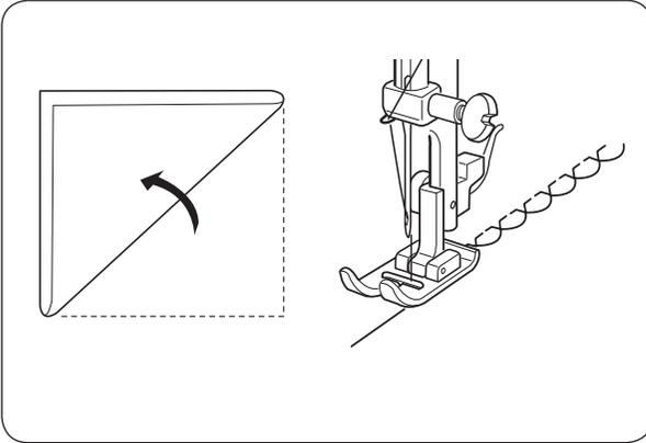
Use a lightweight fabric (tricot, for example). Fold and stitch on the bias. When the needle swings to the right, allow the needle to just clear the folded edge of the fabric. After stitching, open the fabric and iron press the tucks flat to one side.
