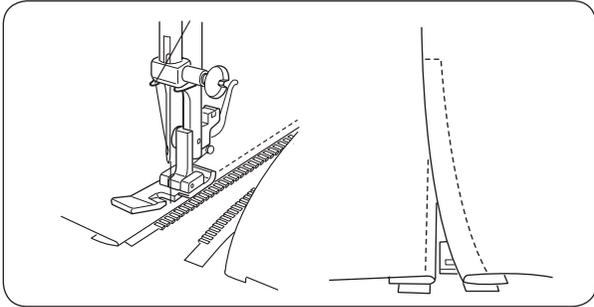
Pin or baste zipper tape to fabric and place it under the foot.
