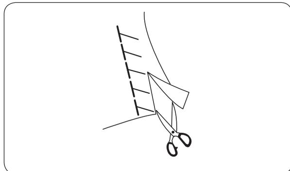
This knit stitch is ideal for sewing swimwear and stretch velour because it provides the greatest amount of elasticity and strength. Place your fabric to allow a 1.6 cm (5/8") seam. Trim the seam allowance after sewing. Be careful not to cut the stitches.
