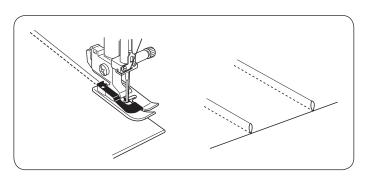
Fold the fabric with the wrong sides together.
