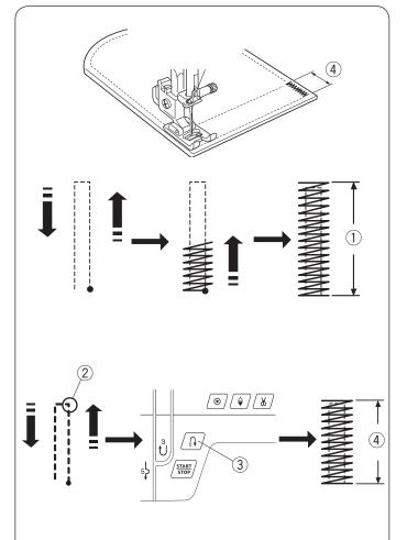
Tacking is used to reinforce pockets, crotches and belt carriers where extra strength is needed.
