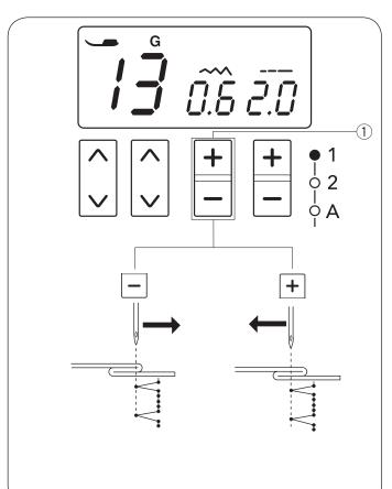
Adjust the needle drop position as follows:
