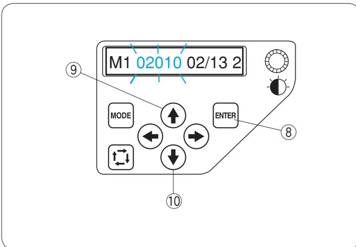
If the thread breaks or runs out while stitching, the machine will automatically stop and the hoop will go back to the position where the thread broke or ran out. However, you can fine-tune the restarting position by moving the hoop.
