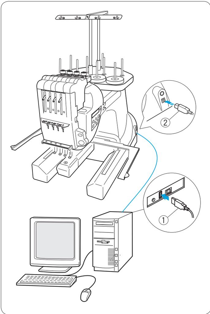
Transfer the embroidery pattern data files between the machine and PC by using optional **Digitizer MB for multi-needle**.
