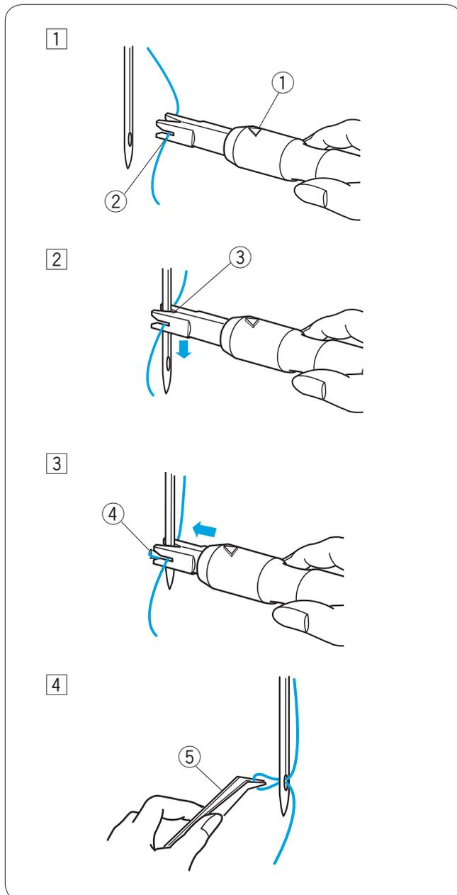
1 Hold the needle threader with a triangle mark facing up. Insert the thread into the Y-notch of the threader from the right.
