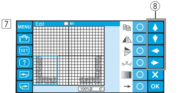
7 Move the flipped pattern to the left bottom corner of the editing screen by using the arrow keys or by dragging it with your fingertip.
