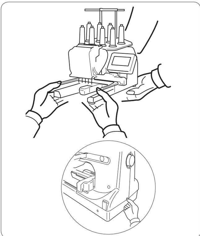
When transporting the machine, be sure it is lifted by two persons. Hold the machine by the two legs and the hand grip on the bottom of the backside of the machine.
