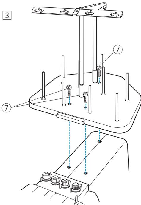
3 Attach the assembled spool stand to the machine with the 3 setscrews (C).
