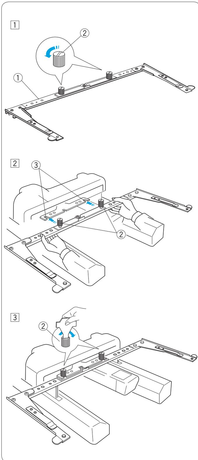
1 Loosen the two thumbscrews on the hoop supporter.
