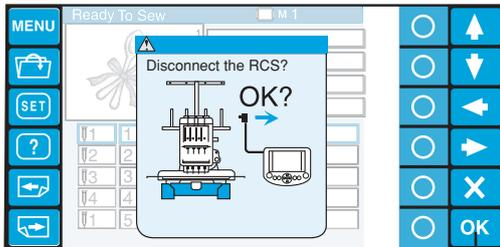
Disconnect the RCS connector from the machine.
