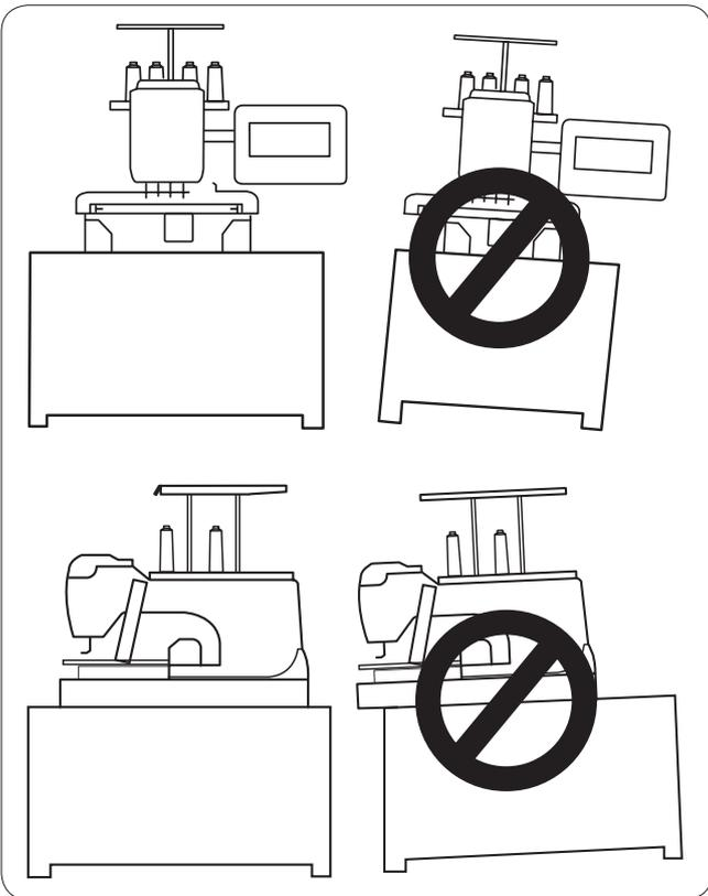
Provide a sufficient space around the machine to allow the hoop to move freely.
