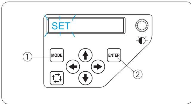
Press the MODE button until the LCD screen shows **SET** blinking.
