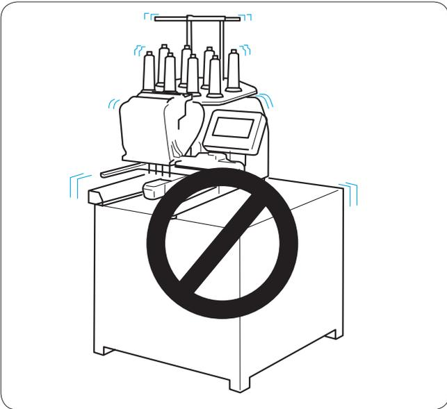
Place the machine on the flat and level surface. Make sure that all the feet firmly contact the surface.
