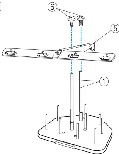
2 Attach the thread guide bar to the thread guide poles with the setscrews (B).
