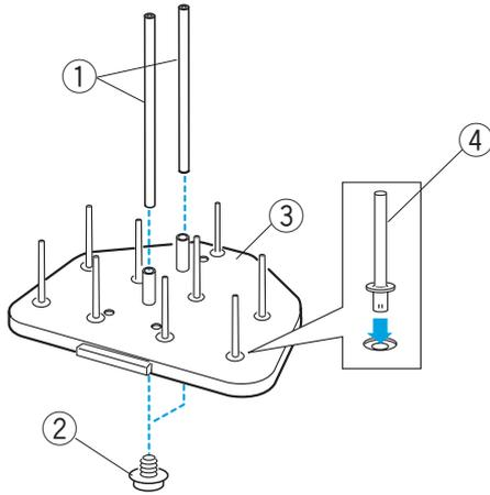
1 Insert the thread guide poles into the sleeve of the spool stand. Secure the poles with setscrews (A) from the bottom.
