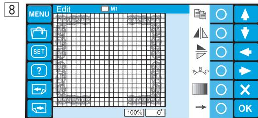
8 Make a duplicate of the pattern and flip it vertically. Move the flipped pattern to the top left corner of the editing screen.
