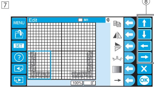
7 Move the flipped pattern to the left bottom corner of the editing screen by using the arrow keys or by dragging it with your fingertip.
