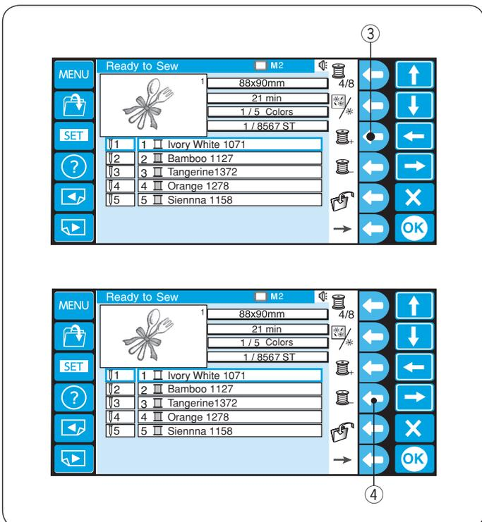
Press the function key next to the previous section (a spool with “-” icon) to select the previous section.
