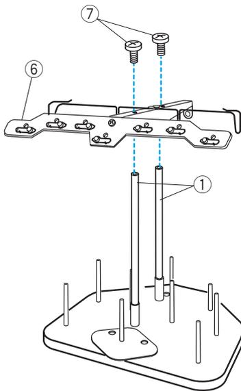
3 Attach the thread guide bar to the thread guide poles with the setscrews B.
