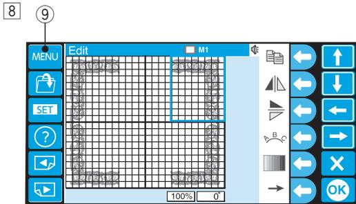
8 Make a duplicate of the pattern and flip it horizontally. Move the flipped pattern to the top left corner of the editing screen.
