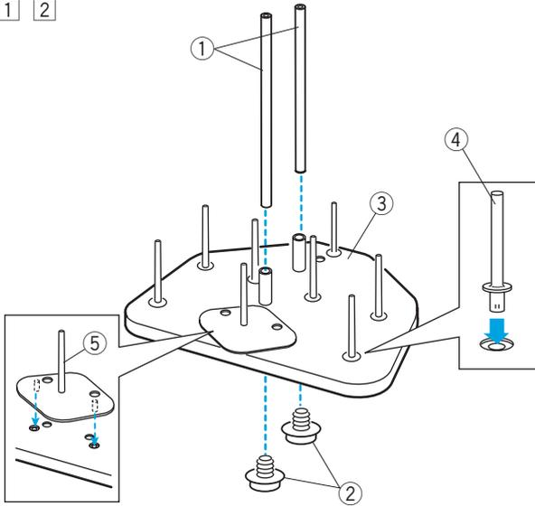
1 Insert the spool pins A into the spool stand.
