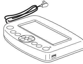
Press the LCD touch panel and buttons gently. Rough or forceful pressing may damage the unit.
