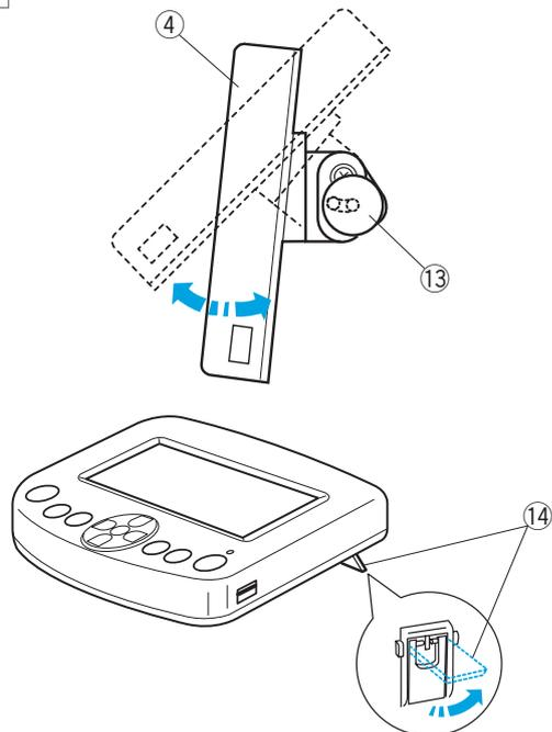
1 Loosen the thumbscrew and open the mounting arm.
