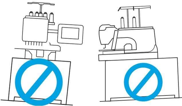
Provide a sufficient space around the machine to allow the hoop to move freely.
