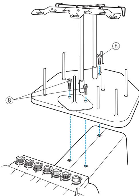
4 Attach the assembled spool stand to the machine with the 3 setscrews.
