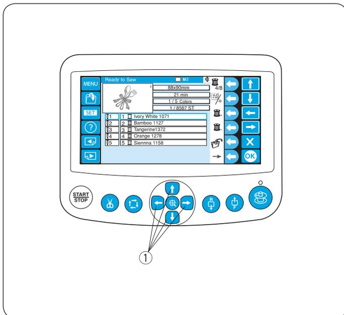
Adjust the hoop position by pressing the jog buttons if necessary.
