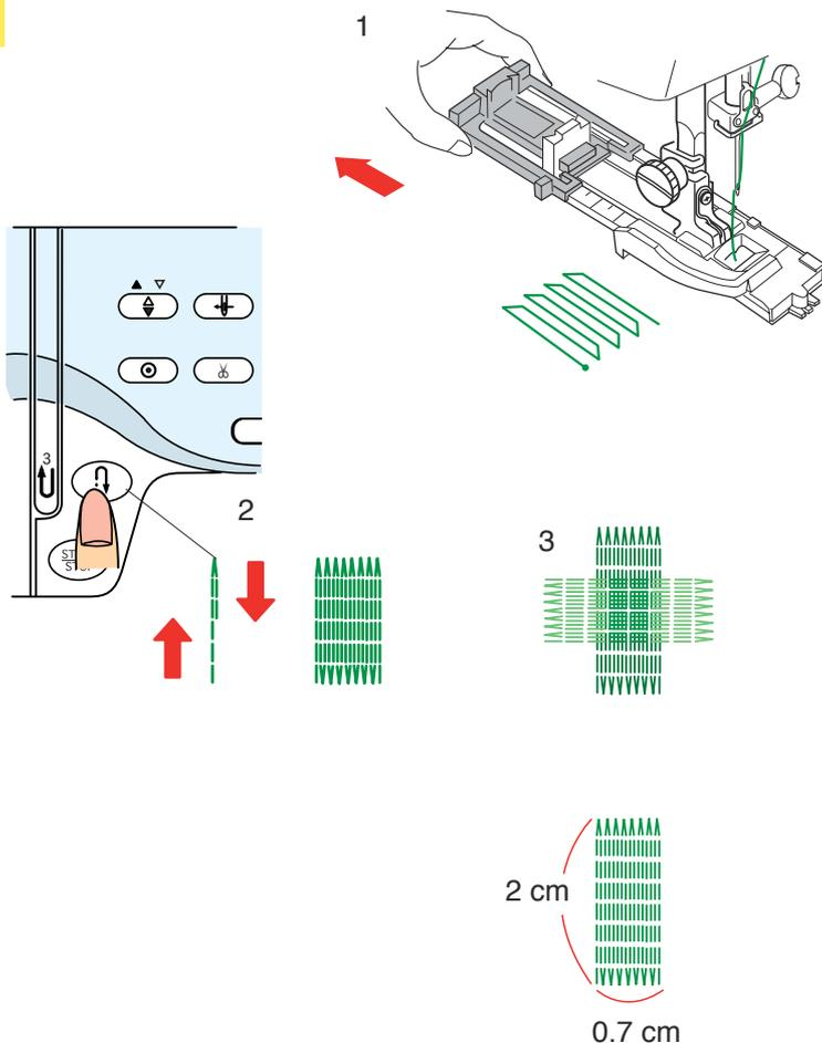
1. Attach the automatic buttonhole foot R and pull the button holder all the way out.
