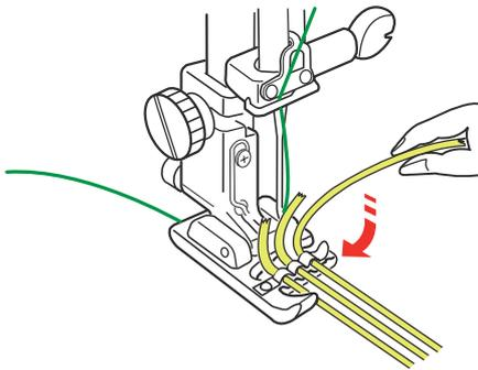
Insert three strands of cording under the spring on the foot. Make sure to pass each strand separately under the spring.
