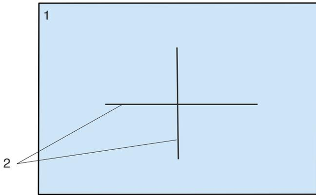
Loosen the hoop tightening screw on the outer hoop. Lay the inner hoop and template on the fabric, matching the centerlines.
