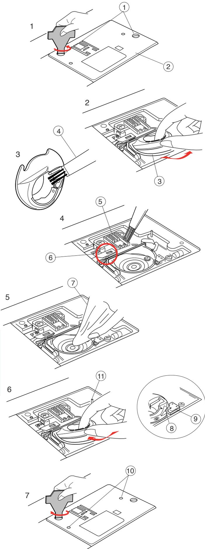
1. Remove the setscrews with the screwdriver key supplied with the machine. Remove the needle plate.
