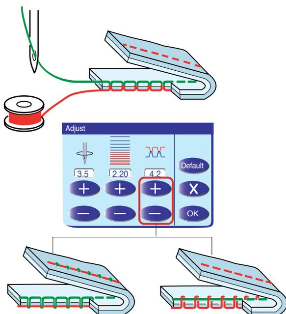
This machine is equipped with the automatic thread tension control, however you may need to manually adjust the tension balance depending on the sewing condition, or you can fine-tune the thread tension to suit your preference.
