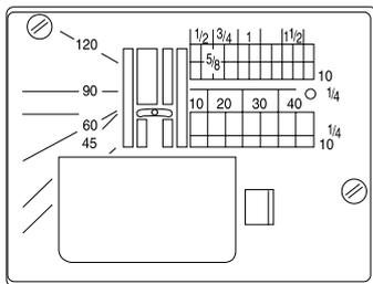
You can seam patchwork pieces at the desired angle without marking, by using the angle scale on the needle plate.
