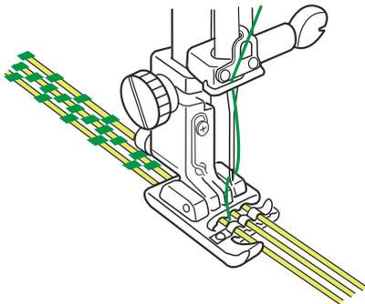
Pull 10 cm (4") of strands under the foot and to the rear. The grooves on the bottom of the foot will hold cording in place while stitching over the cording.
