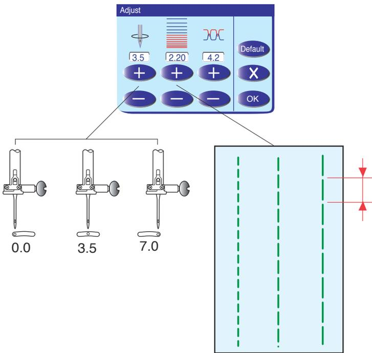
Press the “+” key to move the needle drop position to the right.
