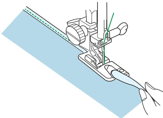
Lower the foot and sew while lifting the edge of the fabric to keep it feeding into the curl smoothly and evenly.
