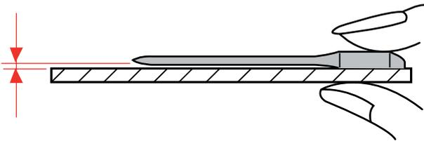
Raise the needle by pressing the up/down needle button and lower the presser foot.
