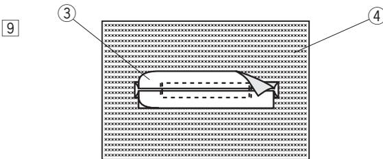
9 The patch should be cut 1 to 1.5 cm (7/16" – 5/8") away from the hole. The corners should be cut rounded off as shown.
