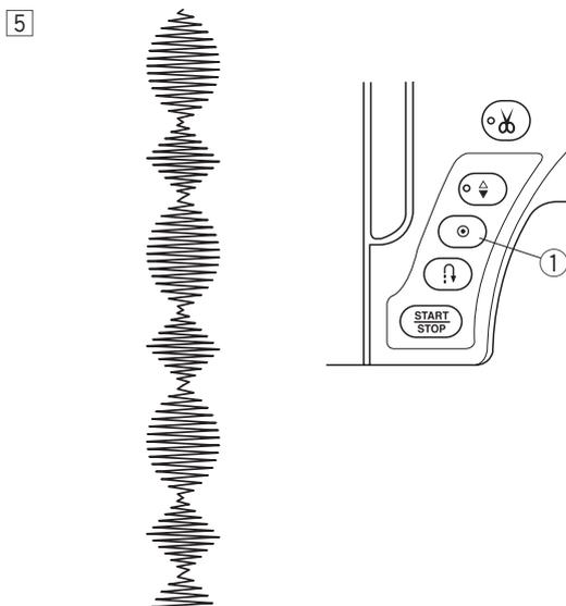
5 Start sewing. Combination of patterns 147 and 151 will be sewn continuously.
