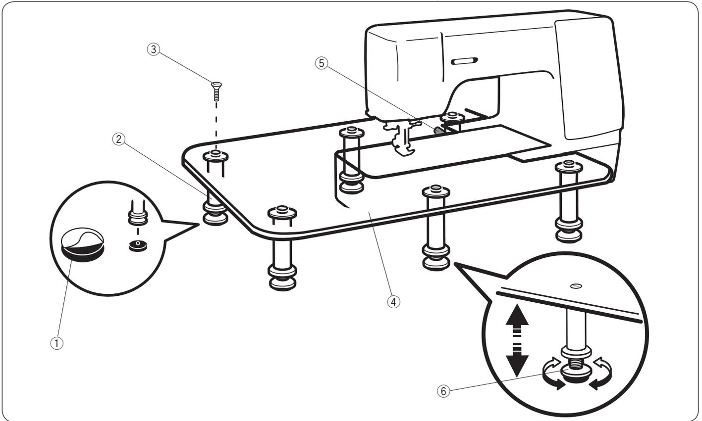
Peel off the backing paper from the rubber soles and attach to the bottom of the legs.
