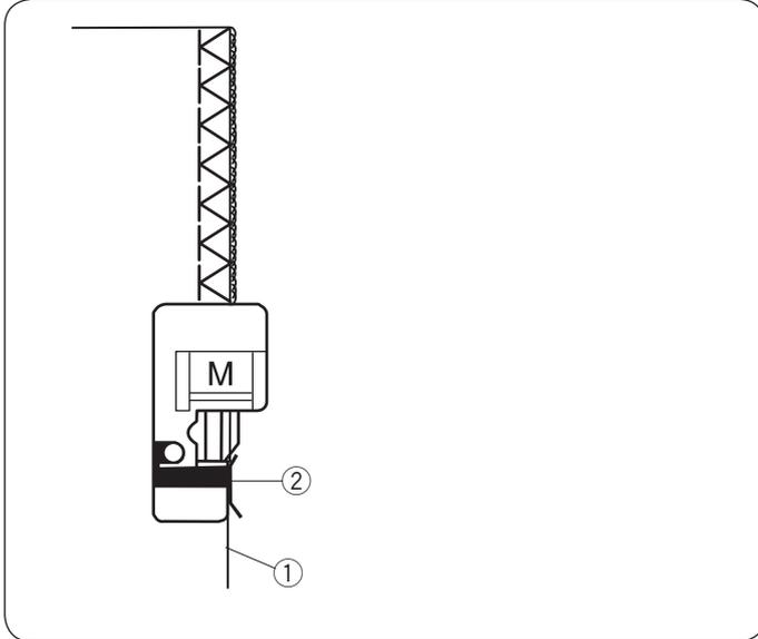
This stitch finishes the edges of fabric similar to a commercial overlocking machine for a professional look. Place the fabric edge next to the guide of the foot and then sew.
