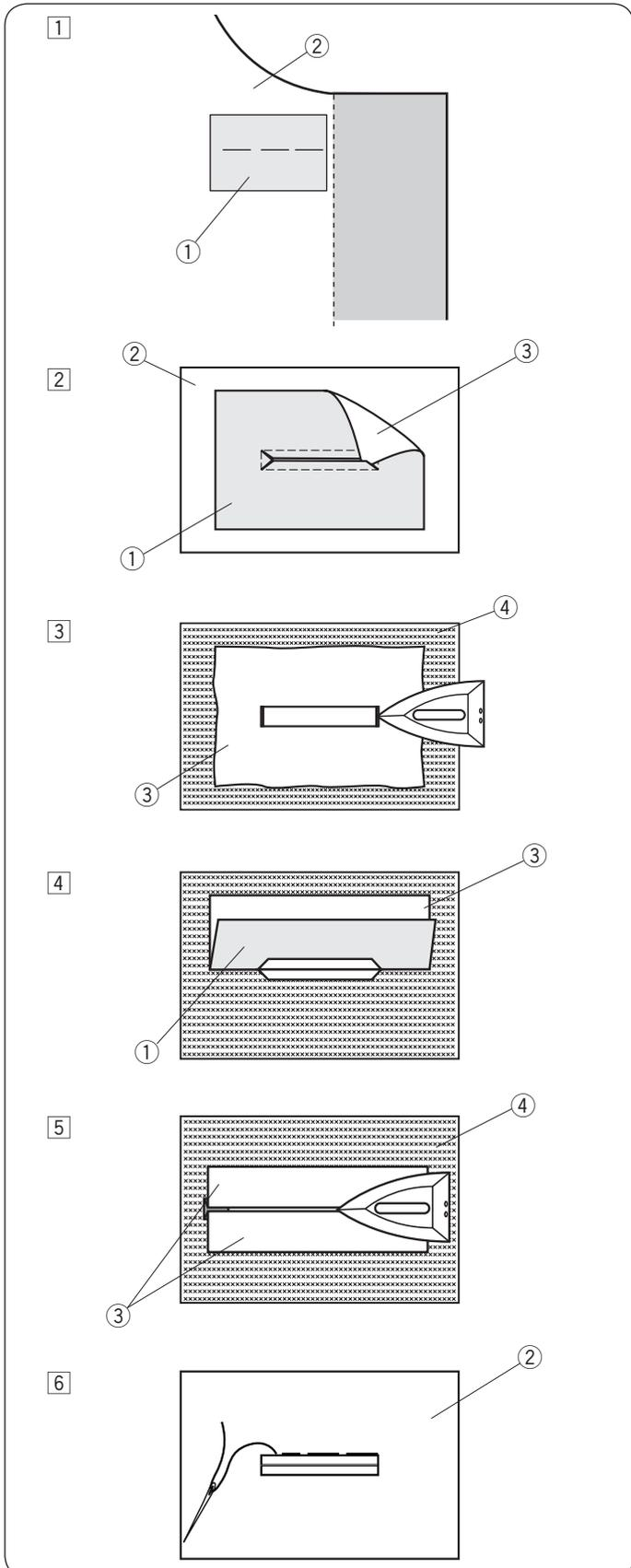
A welted buttonhole is made by stitching a strip or patch of fabric to the buttonhole. Welted buttonholes are particularly suitable for tailored garments, but are not recommended for sheer or delicate fabrics where the patch might show through or add bulk.
