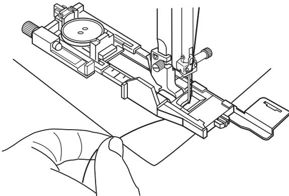
5 Start sewing while pulling the needle thread lightly to the left. After sewing a few stitches, free the thread and continue sewing.
