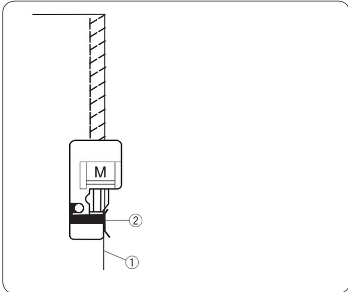
This stitch is recommended for sewing such fabrics as synthetic knits and stretch velour as it provides the greatest amount of elasticity and strength. Place the fabric edge next to the guide of the foot and then sew.
