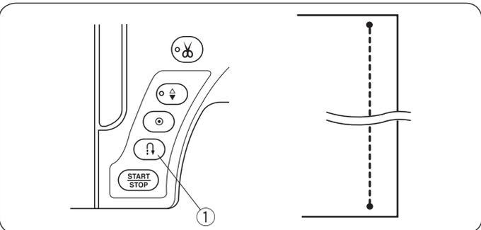
This unique stitch is used where an invisible locking stitch is needed. Lower the needle close to the front edge of the fabric.
