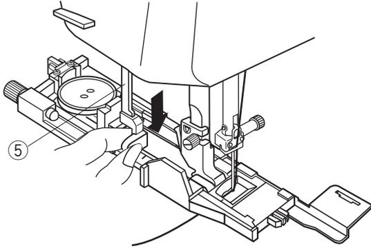
4 Lower the buttonhole foot and pull down the buttonhole lever as far as it will go.
