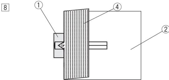
8 Fold over the end of fabric and sew back and forth three times over the triangular end.
