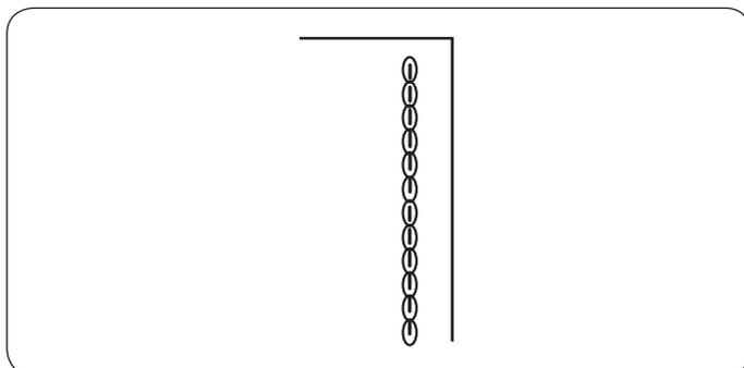
This strong, durable stitch is recommended for areas where both elasticity and strength are needed to ensure comfort and durability. Use it to reinforce areas such as crotch and armhole seams. Also use it when constructing items such as backpacks for extra strength.
