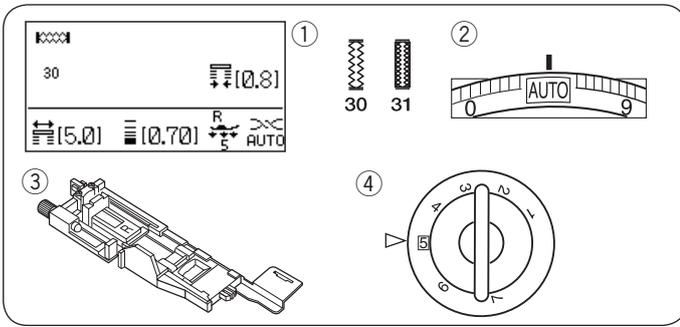
Place the button on the button holder on the buttonhole foot.
