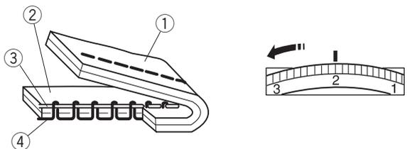
If the needle thread is too loose, the needle thread loops on the underside of the fabric.
