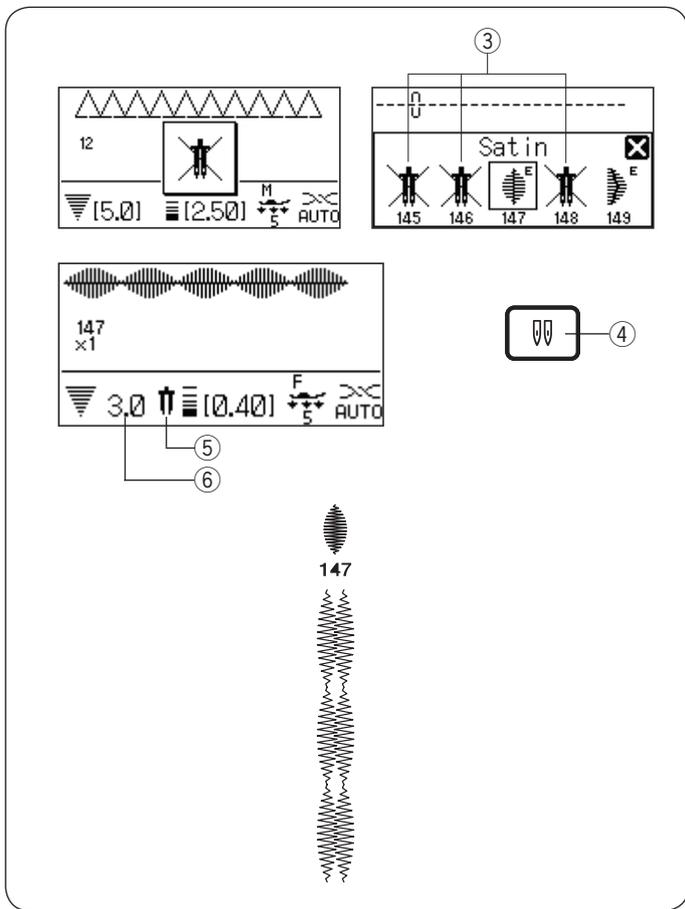
Press the twin needle key and select the desired pattern. Patterns not suitable for twin needle sewing cannot be selected.
