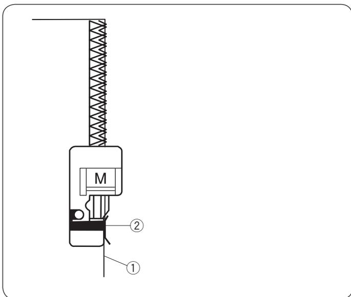
This is an excellent stitch for fabrics that tend to fray extensively such as linens and gabardines. Two rows of zigzag stitches are simultaneously sewn over the edge to insure that fabric will not ravel. Place the fabric edge next to the guide of the foot and then sew.
