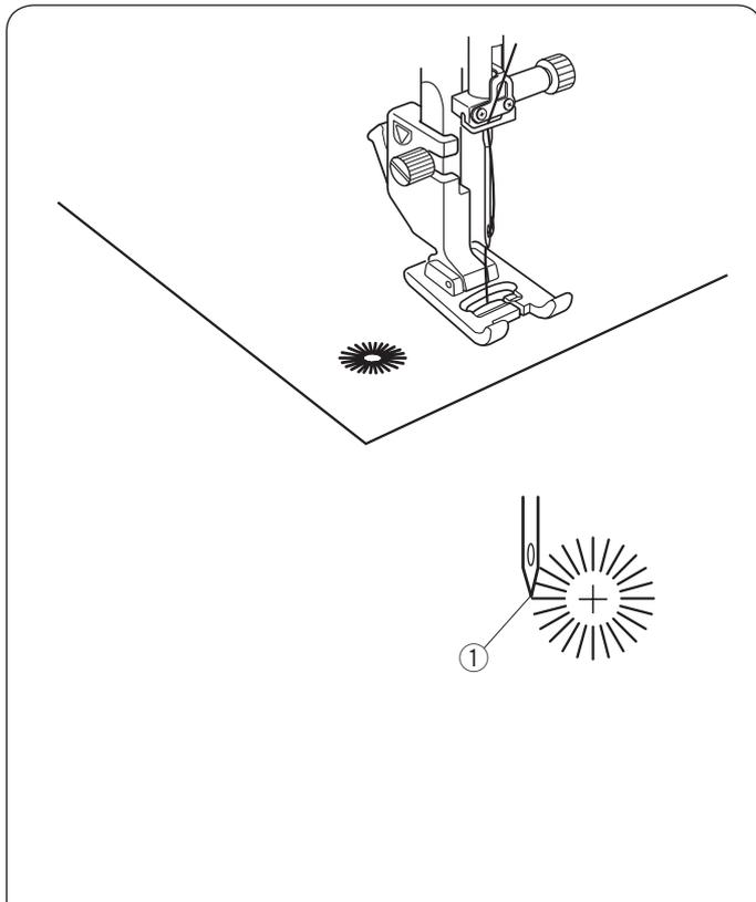
The eyelet is used for belt holes etc.
