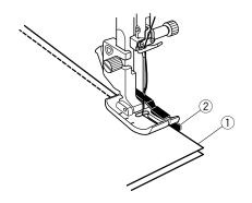
Attach 1/4" seam foot O, which helps you to keep a constant 1/4" (6 mm) seam allowance. Put 2 pieces of fabric with right sides together.
