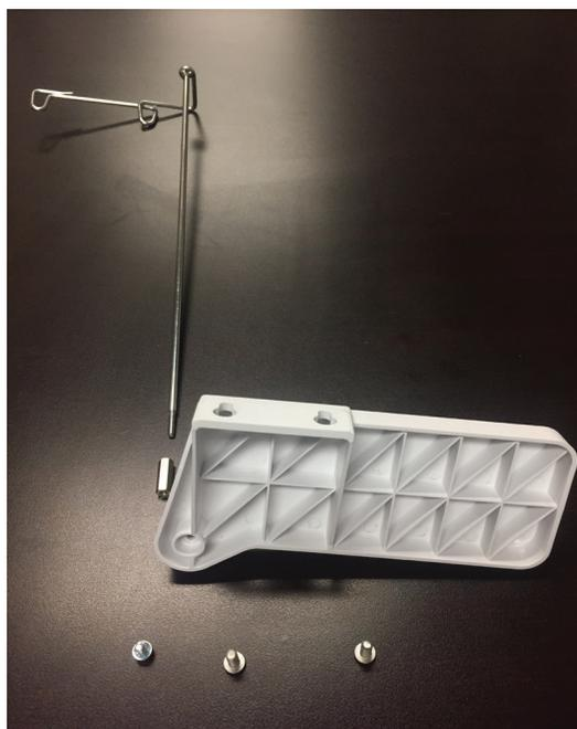
3. Screw the standoff onto the bottom of the thread mast firmly.
