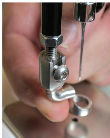
3. Fully tighten the screw with the 2.5 mm hex tool.
