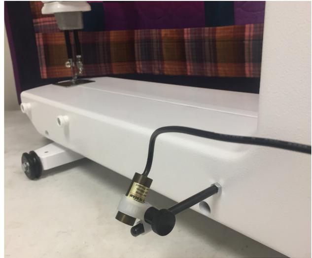
2. Insert the laser stylus into the laser clamp.
