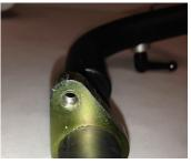
3. Looking through the hole found on the left side of the machine just above the "U" shaped cutout, locate and align the threaded hole on the handlebar bracket.
