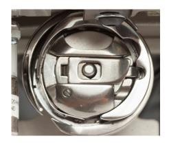
NOTE: Do not insert the bobbin case into the machine by lifting the lever on bobbin case. Use the lever only for removing the bobbin case.
