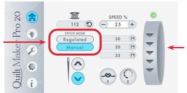
The on-screen hand wheel enables you to rotate the machine's hand wheel from the main screen rather than reaching around the machine to do it manually.
