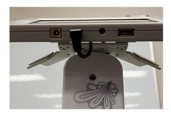
**□ IMPORTANT**: If you have Pro-Stitcher, you will install the Pro-Stitcher tablet computer to the front of the machine instead of the 7-inch display. See the instructions that come with Pro-Stitcher for more information about installing the tablet computer.
