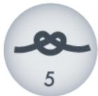
Tie-off button: Use this button to perform a tie-off at the start or finish of your stitching. Touch the button and gently move the machine to perform the micro stitches. The number below the image indicates how many micro stitches will be performed.
