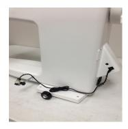
4. Plug the laser cable end into the laser stylus port on the back of the machine. This is found on the tension side of the machine inset in the rectangular shaped opening.
