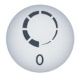
The Easy-Set Tension™ shows the top tension setting as a numeric value on the display. The number on the button indicates the current tension, which is set by manually turning the tension knob. After you establish the tension setting for a particular thread (brand, weight, and color), record the value so you can easily return to that tension setting when using that specific thread again.
