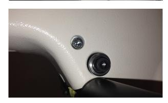
5. Connect the handlebar's USB mini B cables into the side of the machine. Connect the longer cable coming from the handlebar to the bottom connector on the machine and the shorter cable to the closer upper machine connector.
