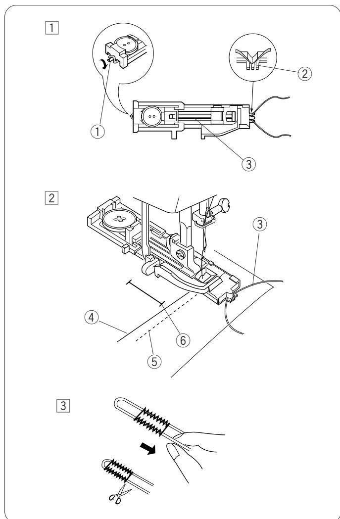
1 With the buttonhole foot raised, hook the filler cord on the spur at the back of the foot.
