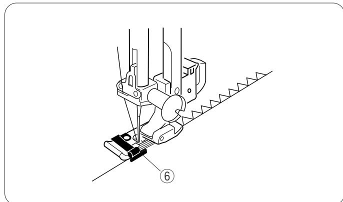
Overcasting is used to prevent fabrics from raveling at raw edges. It can be used to finish a hem edge.
