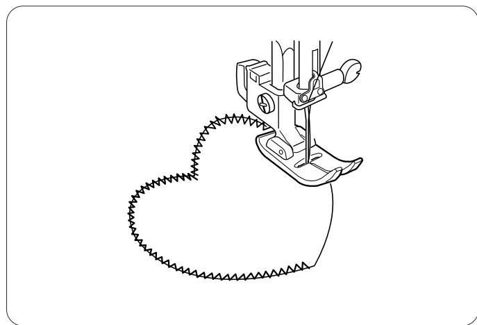
Baste appliquéd pieces on the fabric, or fuse the appliquéd pieces with an iron-on fabric joiner.
