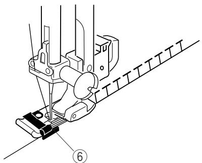
This stitch is ideal for finishing edges of stretch fabrics. It seams and finishes the fabric edges simultaneously.
