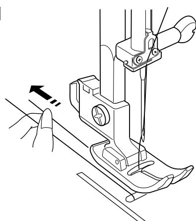
1 Raise the presser foot and hold the needle thread lightly with your left hand.
