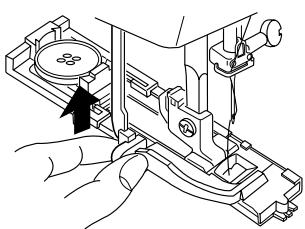
When buttonhole sewing is finished, push the buttonhole lever up as far as it will go.
