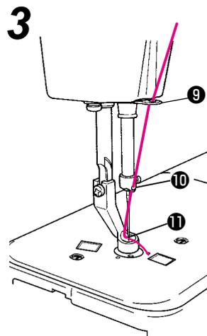
3 ■ Pass the thread through the thread guides 9 and 10. Thread the needle 11.
