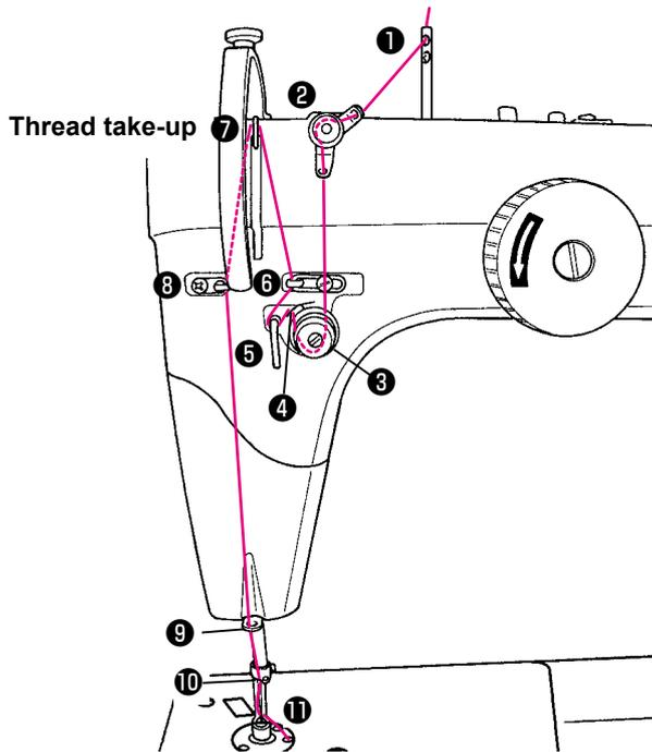
\* Bring the thread take-up (7) to the upper end of its stroke. Then, pass the thread through it.
