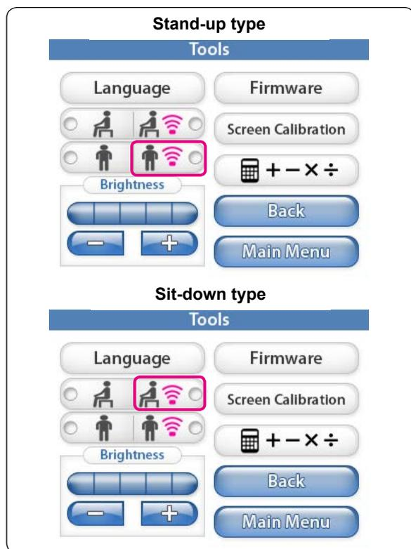
Select the operation usage on the LCD screen operation panel
