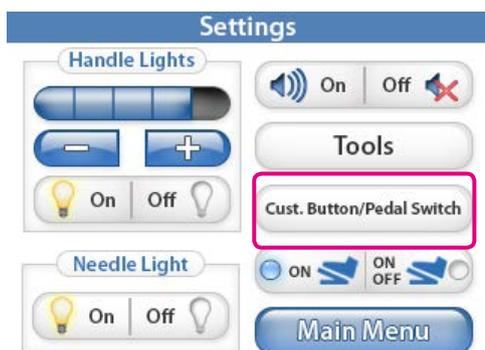
The following functions can be assigned to the left button using the custom switch/pedal switch.
