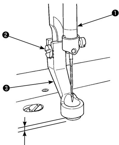
Minimum clearance between the throat plate and the presser foot: 0.5 mm (at the time of shipment)
