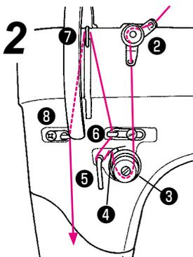
2 ■ Thread the machine head in numerical order, 2 to 8.
