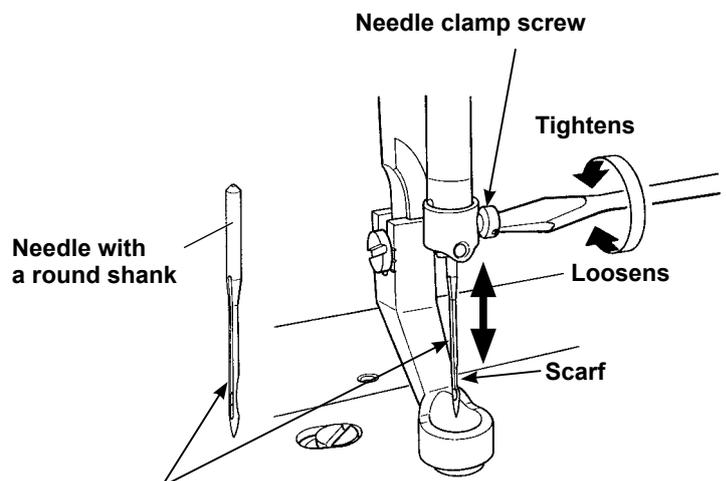
Due to the position of the machine in both the frame and sit down table, the scarf goes to the back and the groove to the front.
