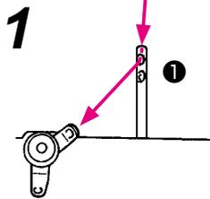
1 ■ Pass the thread through the thread guide 1.
