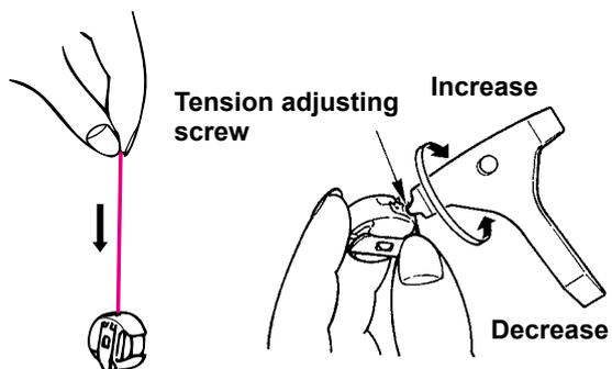
As a measure of the thread tension applied by the bobbin case, when a bobbin (Cotton TEX40) is loaded in the bobbin case, the bobbin should slowly drop by its own weight as illustrated in the figure.
