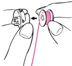
■ Loading the bobbin into the bobbin case.
