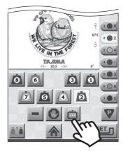
The frame out function is added immediately after the step that was selected in step 1.
