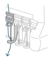
8. Replace the thread pressing shaft and press it down until it clicks into place.
