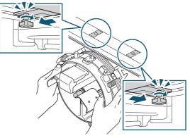
5. Tighten the knobbed screws (two places, at right and left) that were attached in step 2.
