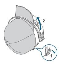
**3.** Open the latches, and remove the fastening band from the cap.
