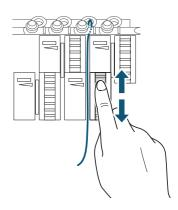
To check the tension of the upper thread, the thread lock needs to be in the raised position as shown below. It cannot be checked properly if the thread lock is not raised.
