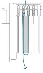
7. As illustrated to the right, thread the upper thread through the needle eye.
