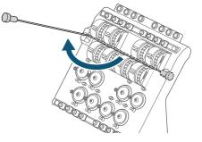
3. Hook the upper thread onto the tip of the upper thread guide (Accessory part), and insert it into the thread tube.
