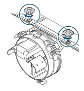
4. Remove the fastening band from the cap frame, and place the backing on the surface of the holder of the cap frame.
