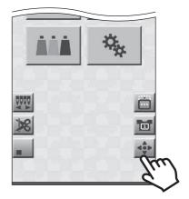
2. Press and hold the relevant arrow icon of the frame travel keys to move the frame to the position you want.
