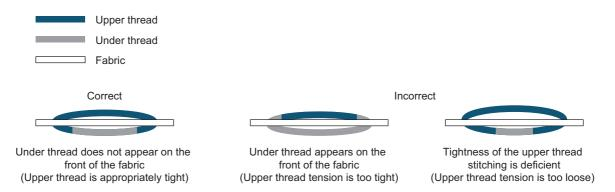
The upper thread tension is raised by turning the thread tension dial upwards. To lower the tension of the upper thread, turn the dial down.
