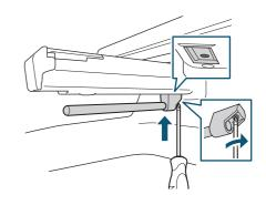
2. Loosely screw in the knobbed screws (two places, at right and left) at the lower part of the frame drive system.
