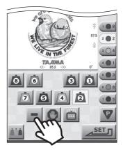
The step repetition operation is added immediately after the step that was selected in step 1. Also, the steps that follow are no longer displayed.
