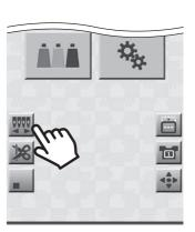
The Manual Color Change screen is displayed. In the color change screen, the needle No. at the current sewing start position is displayed.
