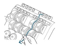
6. As illustrated to the right, place the upper thread on the center thread course of the needle bar case, and then thread it through the hole at the top.
