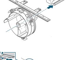
6. Turn the drive ring to move the connecting sashes right and left, so the screw holes in the connecting sashes are lined up with the positions of the screw holes in the moving part (two places, at right and left).
