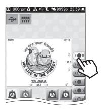
2. Tap the needle No. (1 to 8) that has the thread of the color that you want to assign to step 1.
