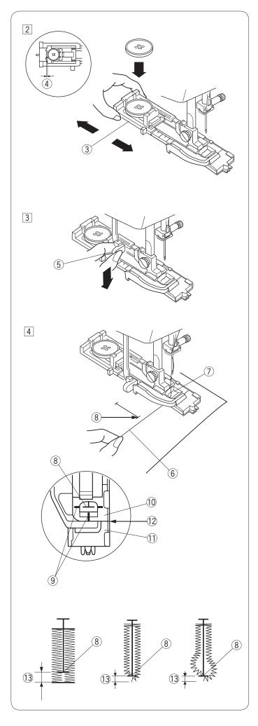
Pull the button holder to the back, and place the button in it. Push it together tightly to the button.
