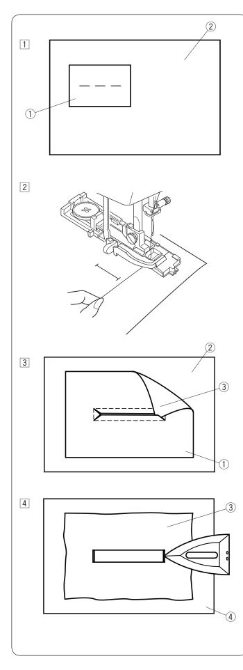
A welted buttonhole is made by stitching a strip or patch of fabric to the buttonhole.
