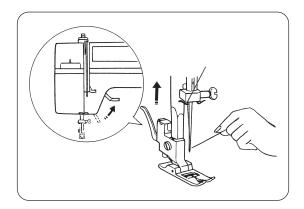
1 Raise the presser foot and hold the needle thread lightly with your hand.
