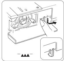
the lever and move it to the direction of arrow as illustrated.
