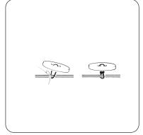
Set the zigzag width dial at " ". Align the both holes of the button with the slot of the foot and place the left hole of the button just below the needle point. Lower the foot and turn the pattern selector until the needle point comes just above the right hole of the button. Sew about five stitches and raise the needle. Set the zigzag width dial at " again and sew a few stitches to lock thread.
