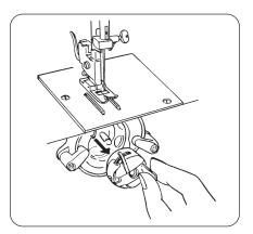
Raise the needle by turning the handwheel toward you.
