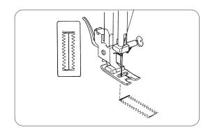
Set the zigzag width dial at " ". Sew a few bartacks and raise the needle from the fabric.
