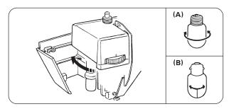
Turn the power switch off before relamping.
