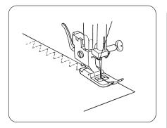
Place the fabric under the presser foot so that the edge will be slightly inside the right hand side of the presser foot.
