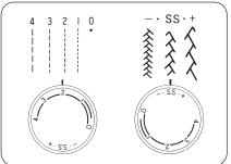
The stitch width for the zigzag stitches ( \geq \text{ and } ), the two needle positions (center and left) for the straight stitch and the triple strength stitch ( | and | ) and buttonhole stitching can be selected with the zigzag width dial.
