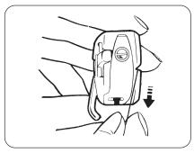
② Pull thread into bobbin case slot.
