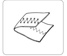
The needle thread and the bobbin thread should interlock in the center of two layers of fabric in straight seams.
