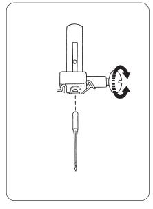
Loosen the needle clamp screw by turning it toward you.
