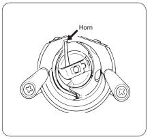
When inserting the bobbin case, place the horn into the recess of the hook race.
