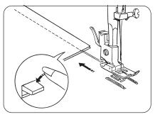
For fastening the ends of seams, press the reverse lever and sew several reverse stitches.
