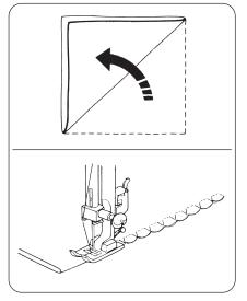
Place the folded edge along the slot of foot.
