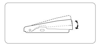
Sewing speed can be varied by the foot control. The harder you press on the control, the faster the machine runs.
