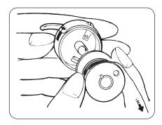
1 Place bobbin into the bobbin case. Make sure the thread unwinds in the direction of arrow.
