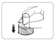
To increase pressure, push down the pressure regulator button until suitable pressure is obtained. To release pressure, push down the ring, then the button will spring up to its highest position.
