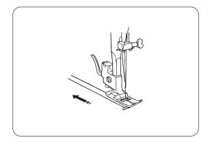
3 Pull 15 cm (6 inches) of both threads back and under the presser foot.
