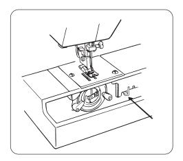
The drop feed lever is located in the hook area.
