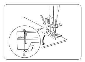
Stop the machine and turn the handwheel toward you to bring the needle down into the fabrics.
