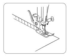
Overedge stitch will be done most successfully when the right side stitches of zigzag fall slightly off the edge of the cloth.
