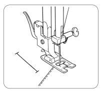
Set the zigzag width dial at Sew down the left side stopping "Im". Slide both threads to the left. Lower the needle into the Raise the needle. garment where the buttonhole is to start, and lower the foot.
