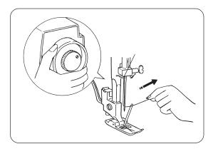
② Turn the handwheel slowly towards you with your right hand until the needle goes down and continue turning the handwheel until the take-up lever is at its highest position. Lightly draw up the needle thread forming a loop of the bobbin thread.
